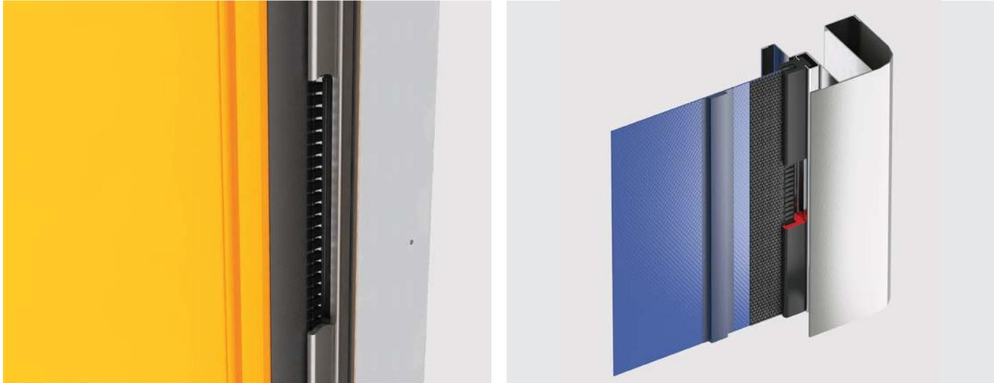
Door curtain is made without any rigid pieces, making them safe for use by equipment and staff. DoorHan high-speed doors are self-repairing, meaning that if door curtains come off of their track (for example, in the event of impact with a forklift) the system will automatically guide the curtain back into the track on the next cycle.
