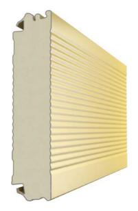
Sandwich panel. Is made of aluminium thikness 0.7 mm with PU foam inside. Dimensions : 185x40mm
